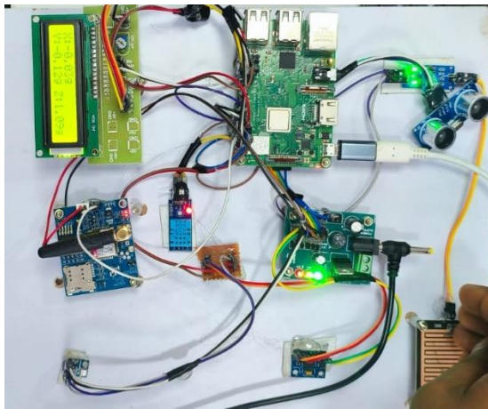
FIG1- Proposed IoT-Based Multi-Sensor Monitoring System Architecture
