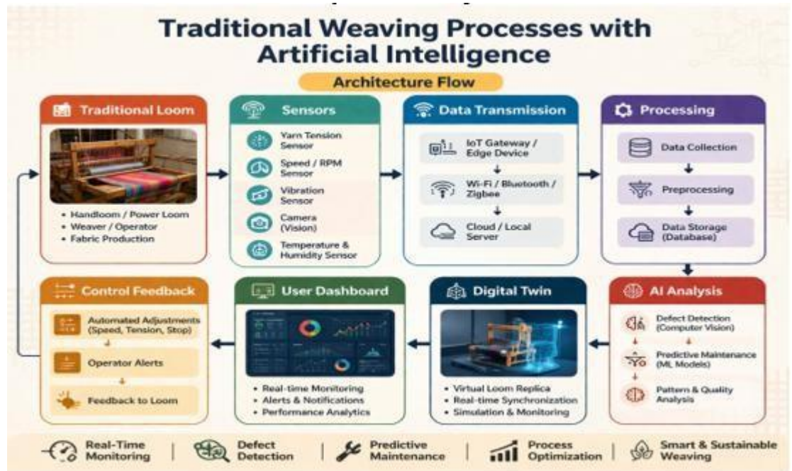
Fig 1: The Architecture Traditional Weaving Processes with Artificial Intelligence
